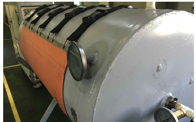
Picture 4. Foil type jacket heater Model FBJH-SR/Y6000F
